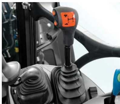
24x24 Dual Command™ gearshift lever with hi-lo buttons on side
